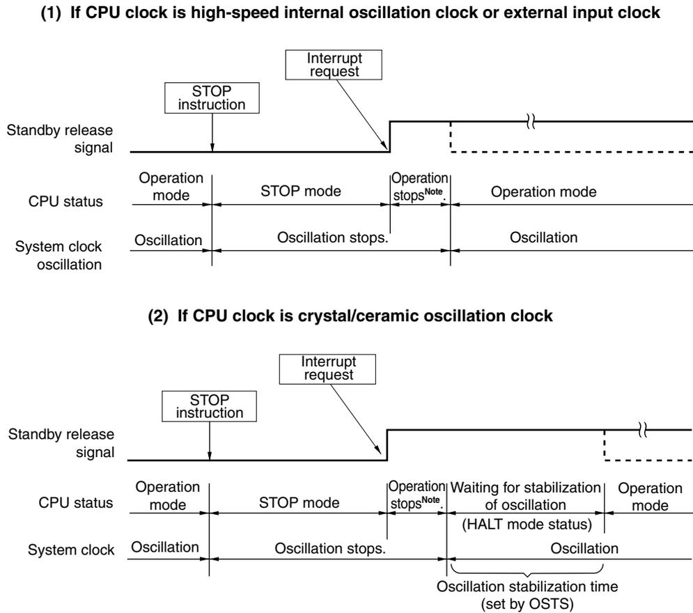
**Note** The operation stop time is 17  $\mu s$  (MIN.), 34  $\mu s$  (TYP.), and 67  $\mu s$  (MAX.).
