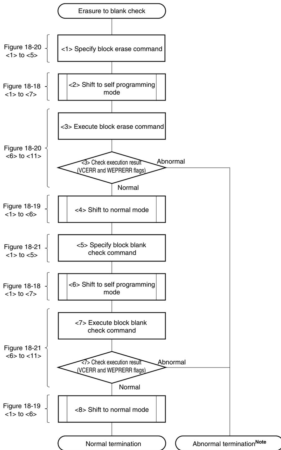
**Note** Perform processing to shift to normal mode in order to return to normal processing.
