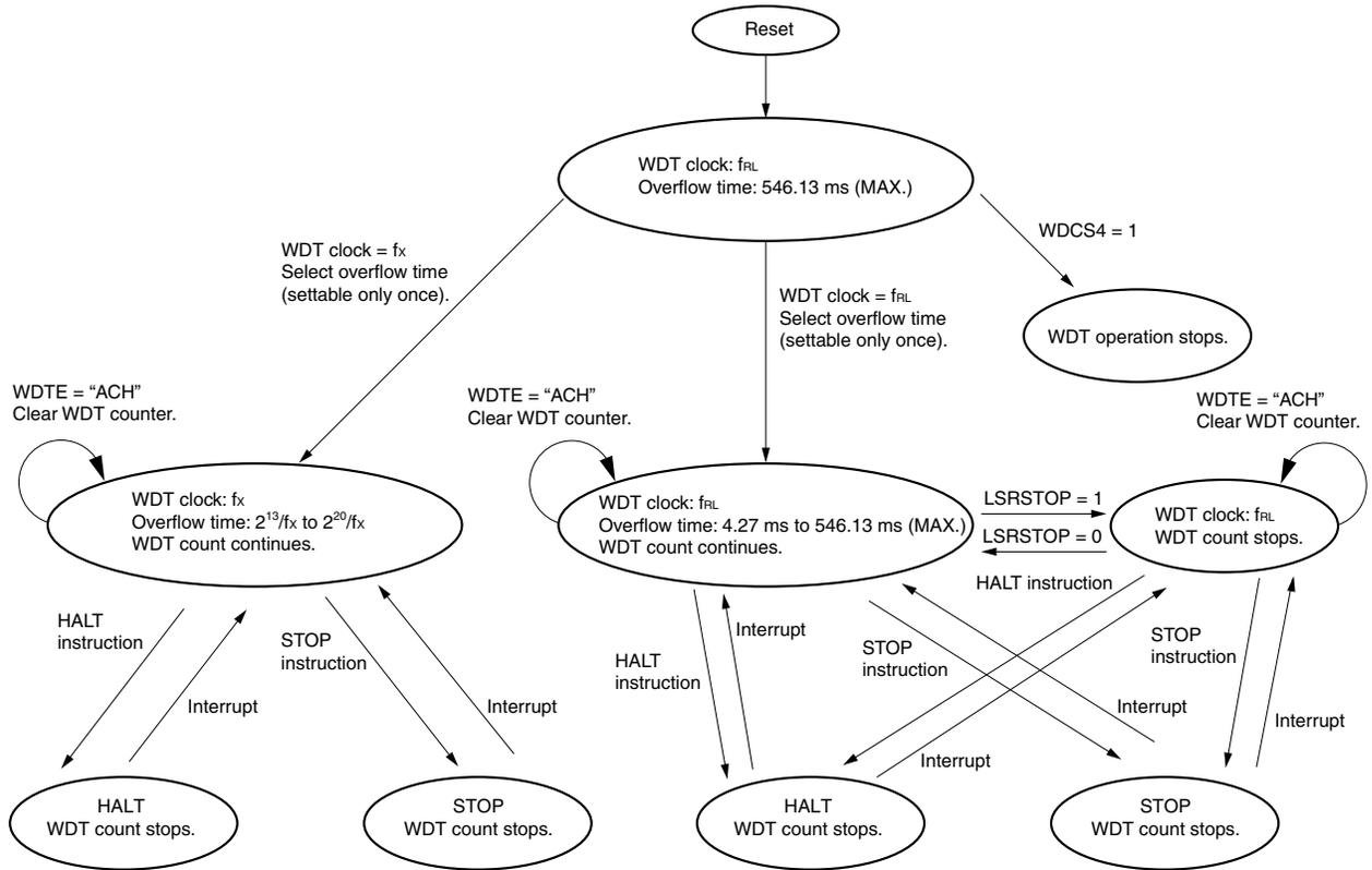
**9.4.3 Watchdog timer operation in STOP mode (when “low-speed internal oscillator can be stopped by software” is selected by option byte)**
