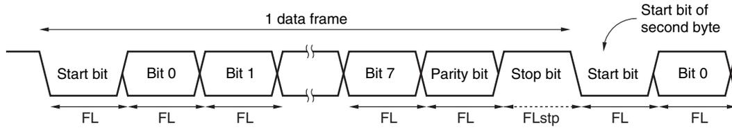
Where the 1-bit data length is  $FL$ , the stop bit length is  $FL_{\text{stp}}$ , and base clock frequency is  $f_{\text{CLK6}}$ , the following expression is satisfied.
