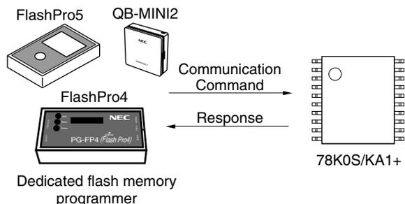
Communication commands are listed in the table below. All these communication commands are issued from the flash memory programmer and the 78K0S/KA1+ performs processing corresponding to the respective communication commands.
