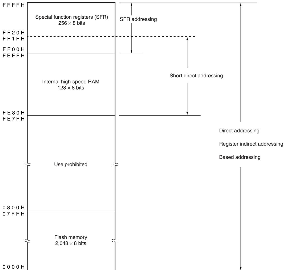
Figure 3-4. Data Memory Addressing ( $\mu$ PD78F9222)
