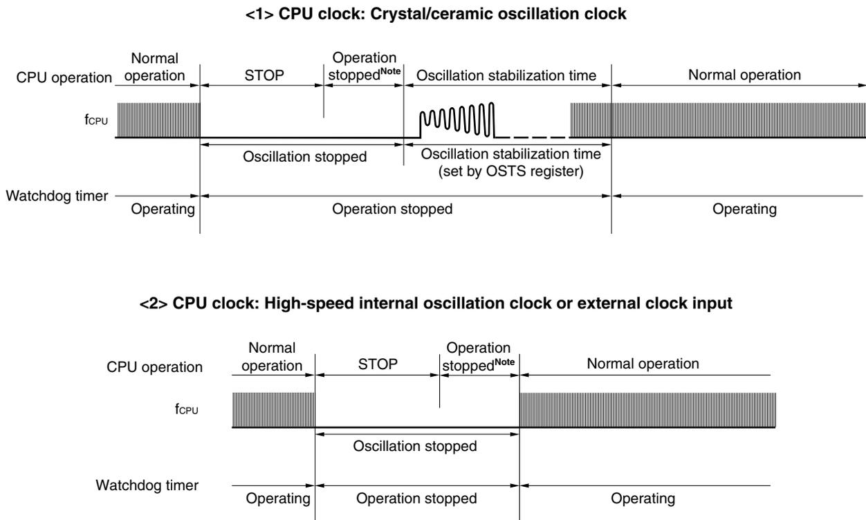
**Note** The operation stop time is 17  $\mu\text{s}$  (MIN.), 34  $\mu\text{s}$  (TYP.), and 67  $\mu\text{s}$  (MAX.).
