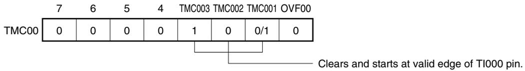
**Note** If the valid edge of TI000 pin is specified to be both the rising and falling edges, 16-bit timer capture/compare register 000 (CR000) cannot perform the capture operation.
