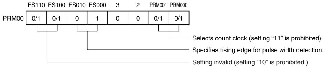
**(c) 16-bit timer mode control register 00 (TMC00)**
