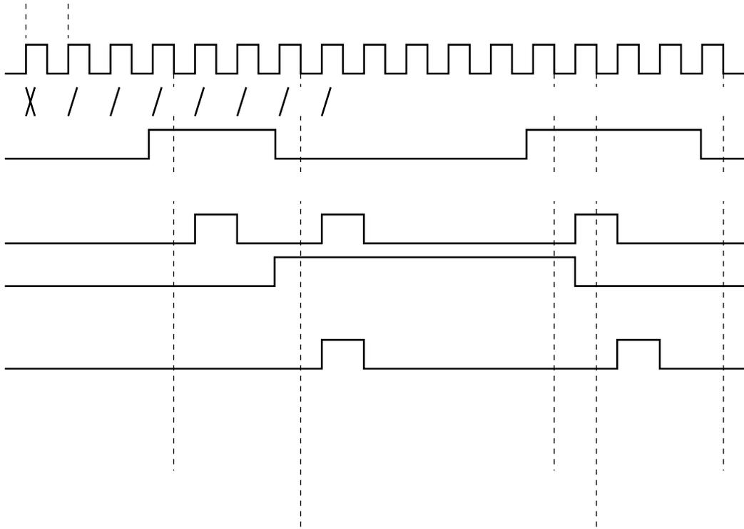
**Figure 6-23. Control Register Settings for Pulse Width Measurement with Free-Running Counter and Two Capture Registers (with Rising Edge Specified)**
