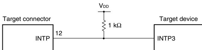
**Figure 19-3. Circuit Connection for the Case Where QB-MINI2 Is Used Only for Programming**
