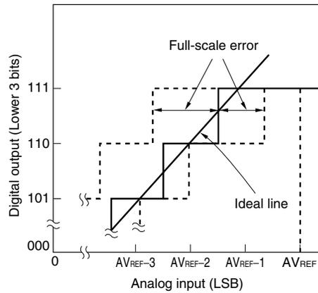
**Figure 10-17. Integral Linearity Error**
