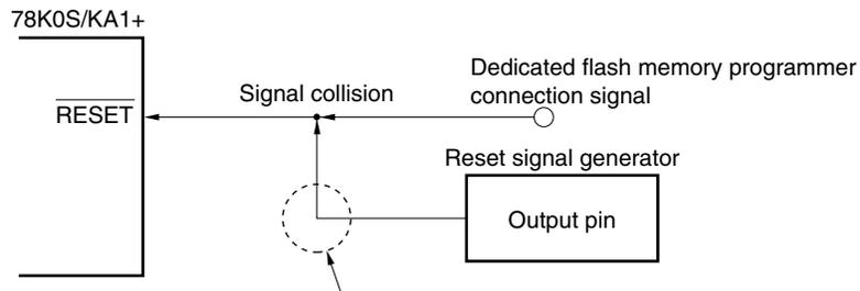
In the flash memory programming mode, the signal output by the reset signal generator collides with the signal output by the dedicated flash memory programmer. Therefore, isolate the signal of the reset signal
