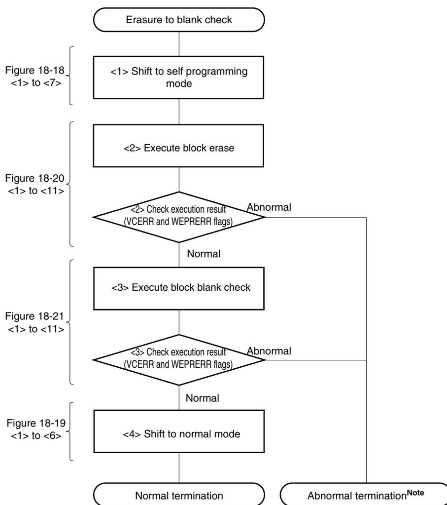
**Note** Perform processing to shift to normal mode in order to return to normal processing.
