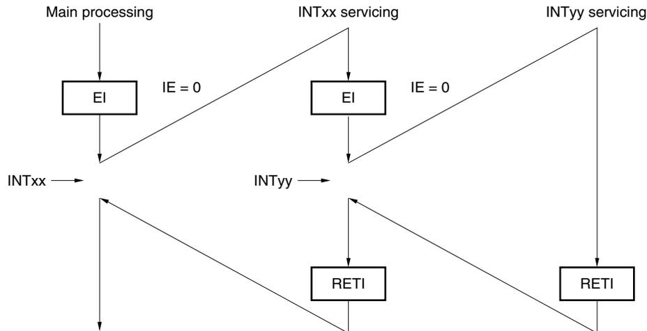
During interrupt INTxx servicing, interrupt request INTyy is acknowledged, and multiple interrupts are generated. Before each interrupt request acknowledgment, the EI instruction is issued, the interrupt mask is released, and the interrupt request acknowledgment enable state is set.
