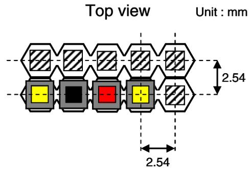
□ : A interval pin header → More than 2.54mm
