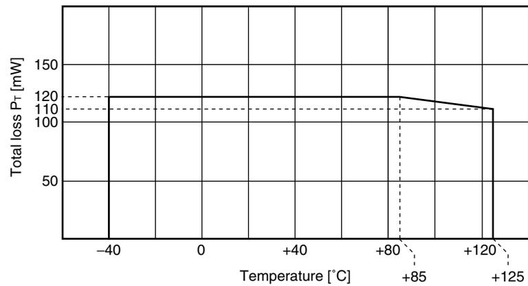
Use the following formula to perform design such that the sum of the power consumption of the device is less than or equal to the total loss  $P_T$  (use at 80% or less of the rated value is recommended).
