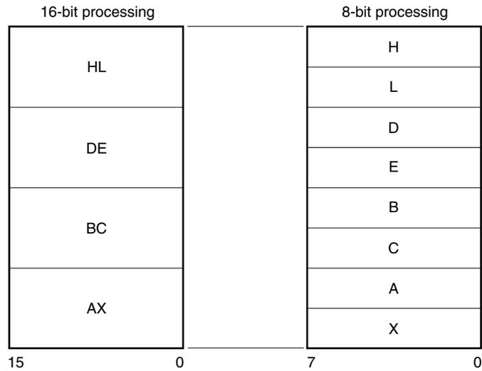
**Figure 3-10. General-Purpose Register Configuration (2/2)**
