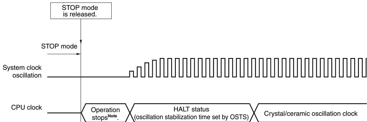
**Note** The operation stop time is 17  $\mu$ s (MIN.), 34  $\mu$ s (TYP.), and 67  $\mu$ s (MAX.).
