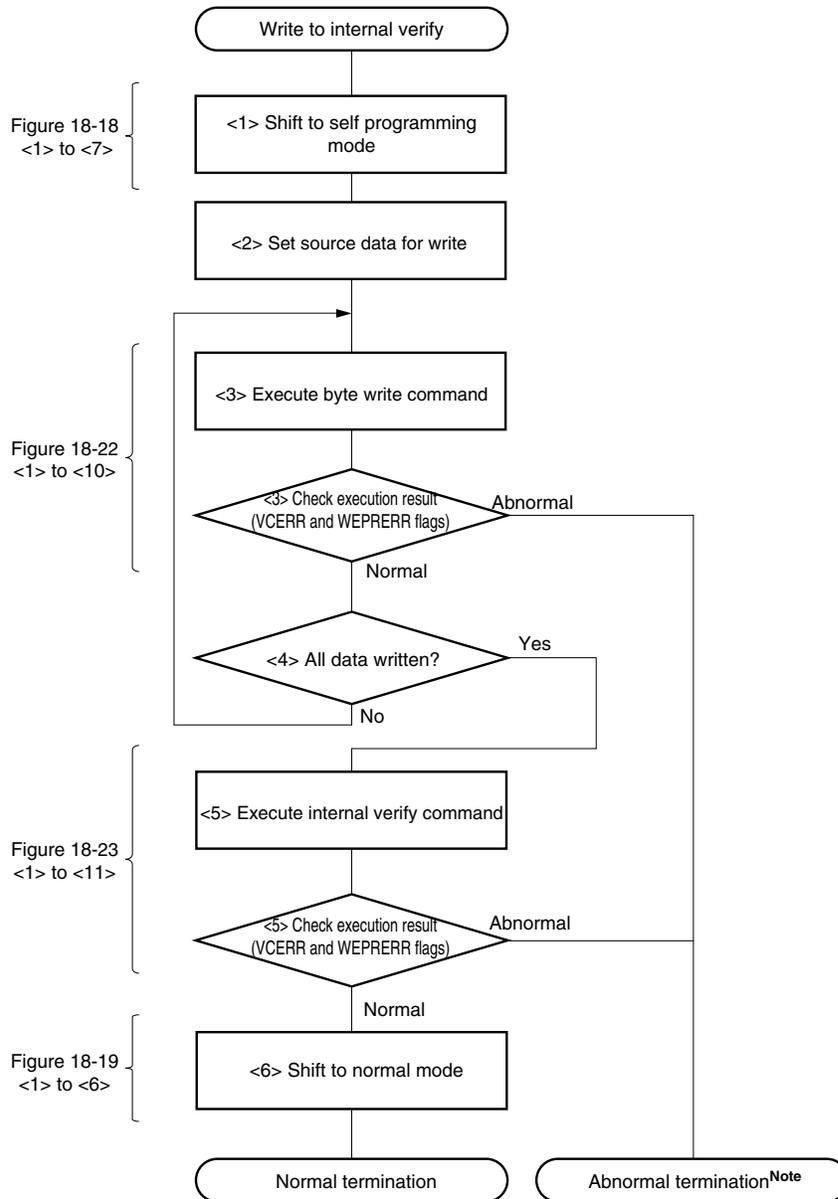
**Note** Perform processing to shift to normal mode in order to return to normal processing.
