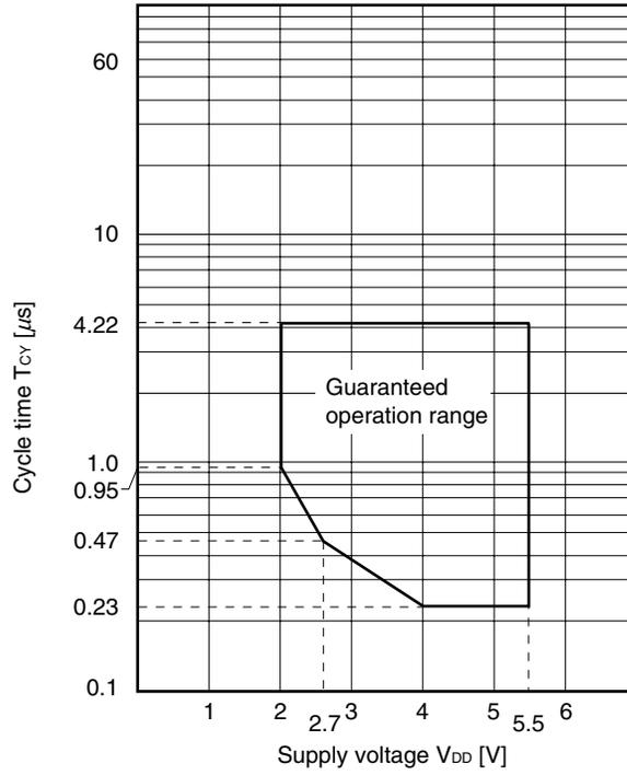
(2) Serial interface ( $T_A = -40$  to  $+85^\circ\text{C}$ ,  $V_{DD} = 2.0$  to  $5.5\text{ V}^{\text{Note}}$ ,  $V_{SS} = 0\text{ V}$ )
