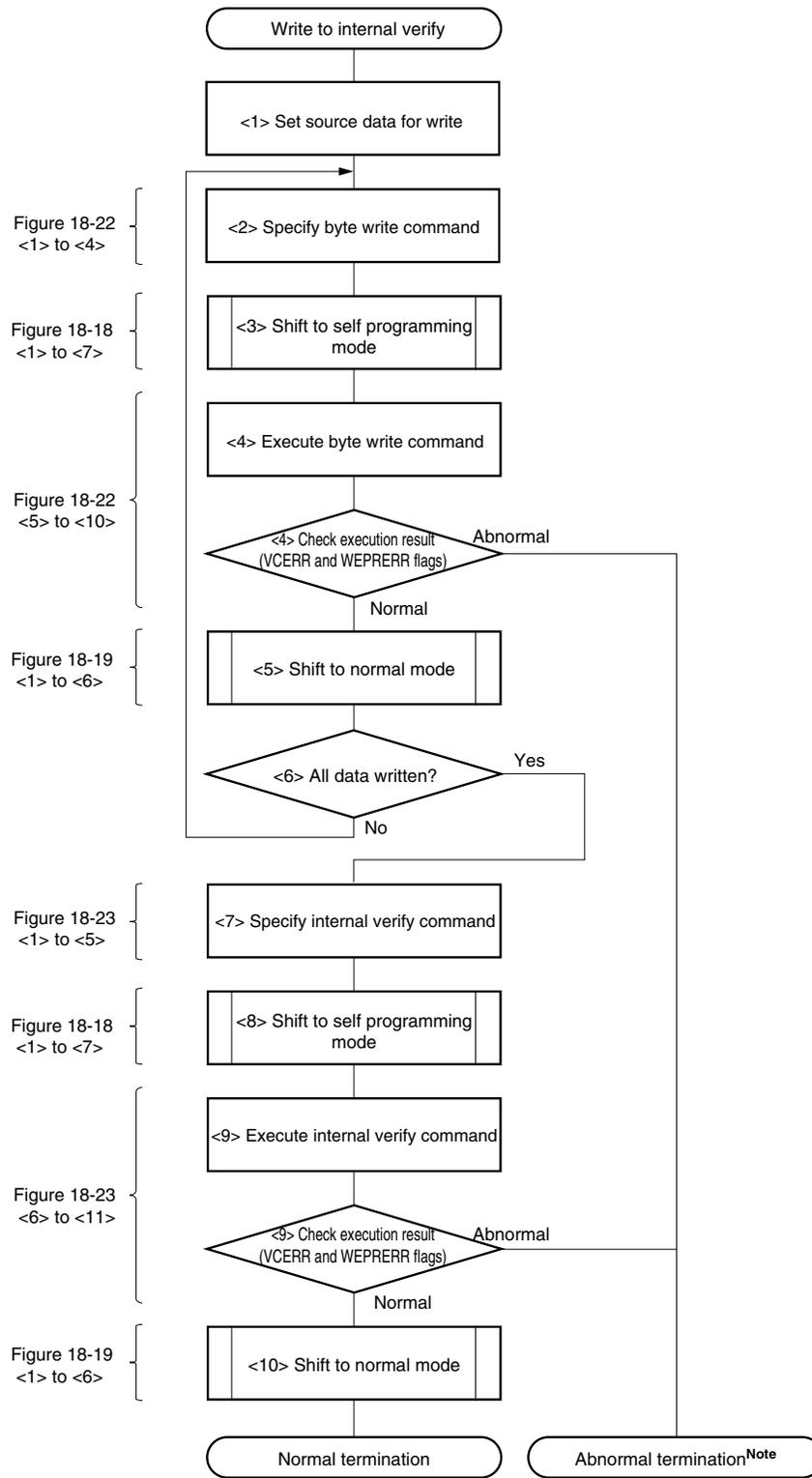
**Note** Perform processing to shift to normal mode in order to return to normal processing.
