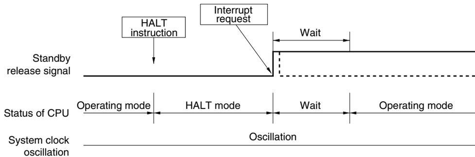
**Remarks 1.** The broken lines indicate the case when the interrupt request which has released the standby mode is acknowledged.
