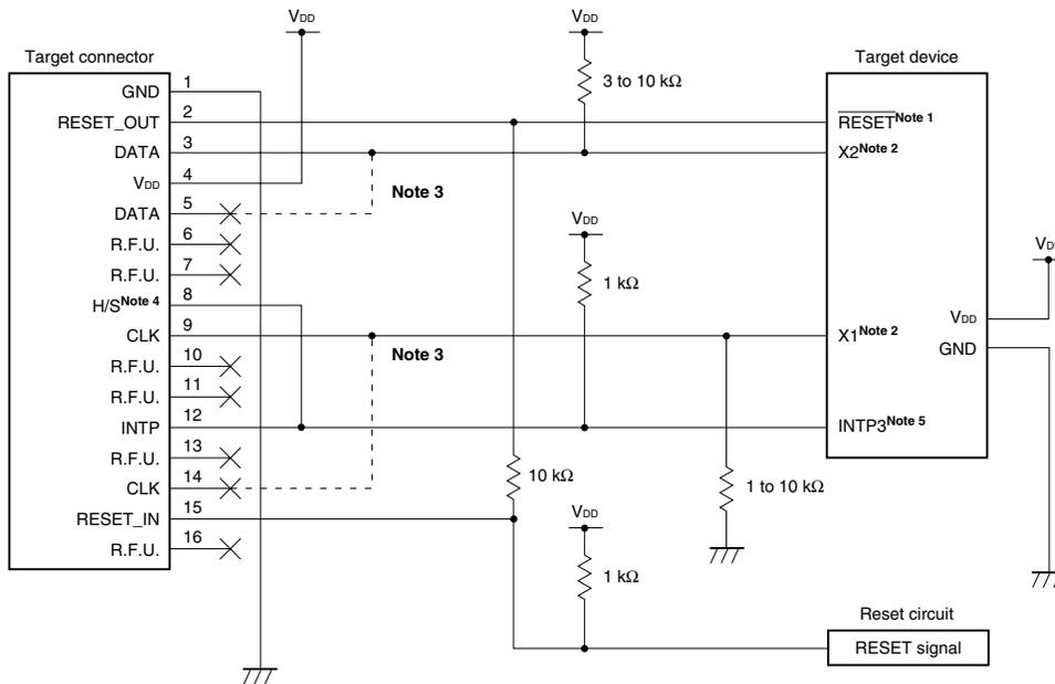
**Caution** The constants described in the circuit connection example are reference values. If you perform flash programming aiming at mass production, thoroughly evaluate whether the specifications of the target device are satisfied.
