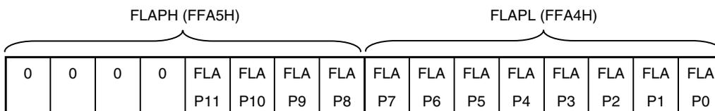
**Caution** Be sure to clear bits 4 to 7 of flash address pointer H (FLAPH) and flash address pointer H compare register (FLAPHC) to 0 before executing the self programming command. If the self programming command is executed with these bits set to 1, the device may malfunction.
