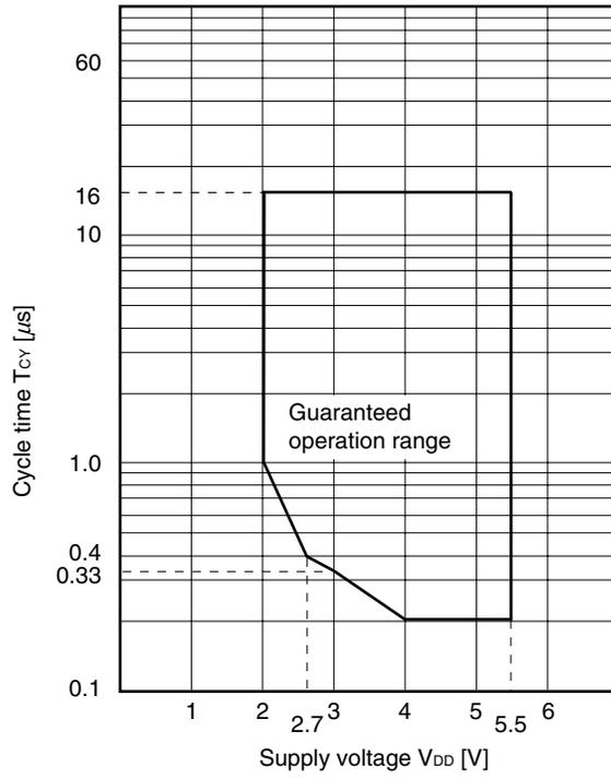
**$T_{CY}$  vs.  $V_{DD}$  (High-Speed Internal Oscillation Clock)**
