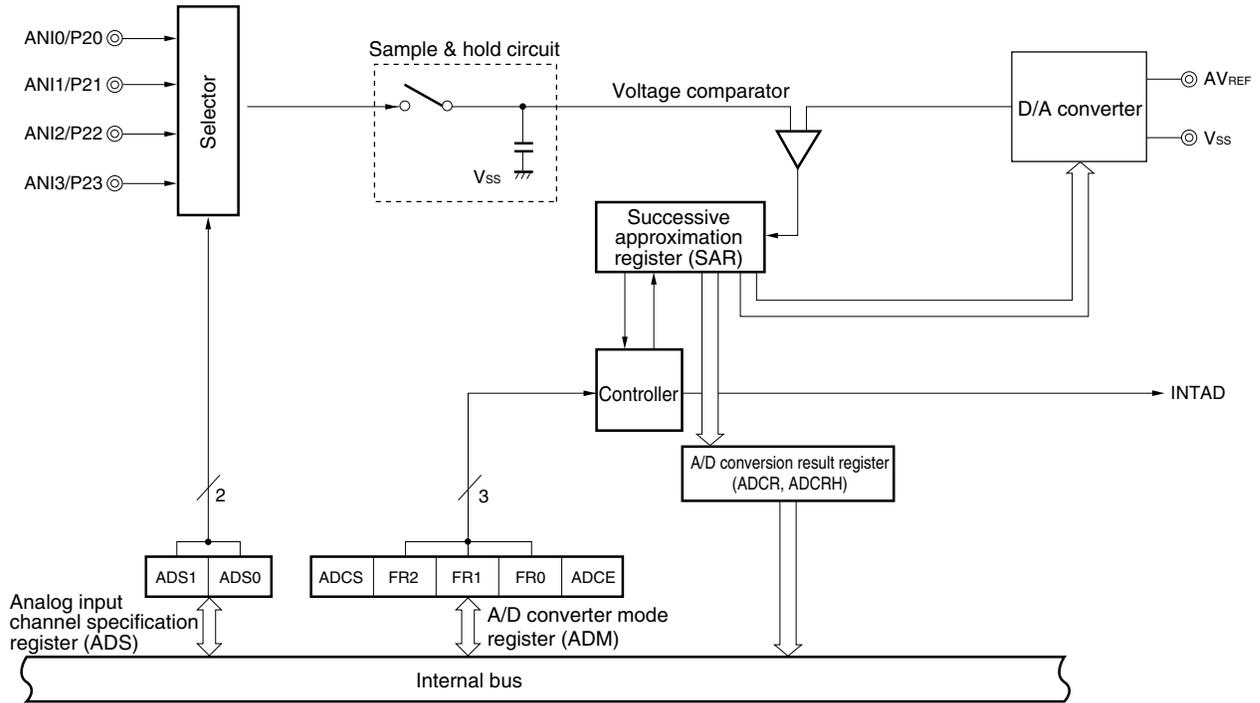
**Caution** In the 78K0S/KA1+, V<sub>SS</sub> functions alternately as the ground potential of the A/D converter. Be sure to connect V<sub>SS</sub> to a stabilized GND (= 0 V).
