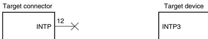
**Figure 19-4. Circuit Connection for the Case Where QB-MINI2 Is Used for Debugging and Debugging of INTP3 Pin Is Performed Only with Real Machine**
