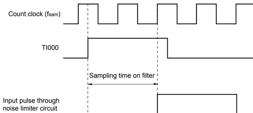
**Remark** The count clock ( $f_{sam}$ ) can be selected using bits 0 and 1 (PRM000, PRM001) of prescaler mode register 00 (PRM00).
