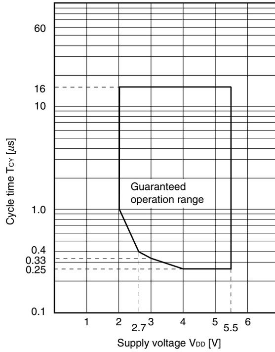
**$T_{CY}$  vs.  $V_{DD}$  (High-Speed Internal Oscillation Clock)**
