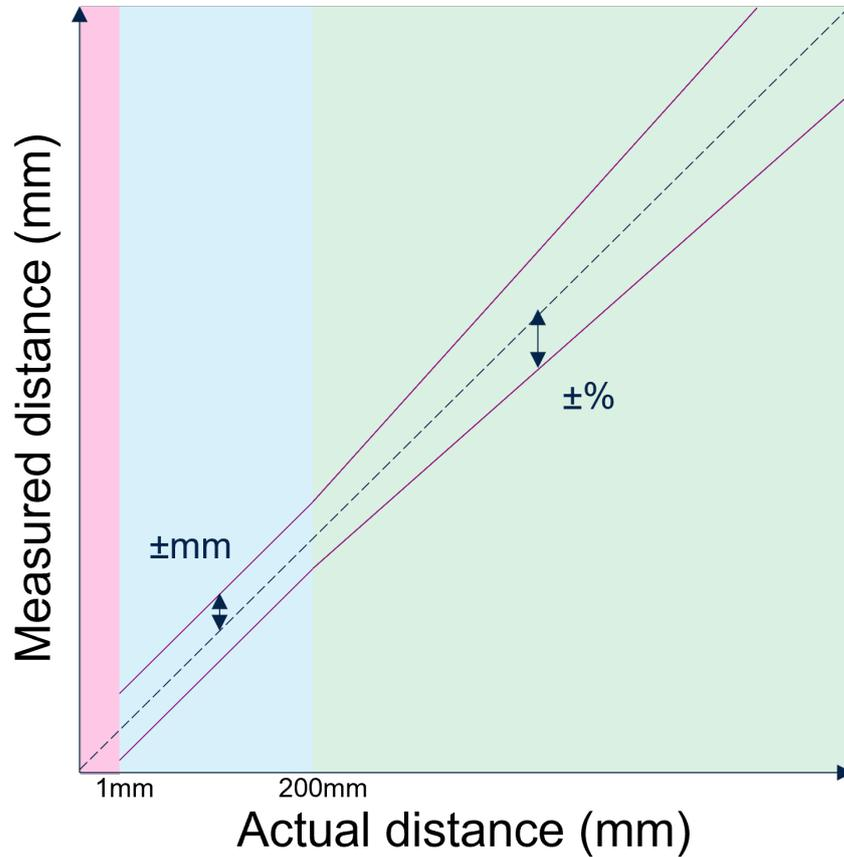
The ranging accuracy is a direct evaluation of the measurement error, including offset errors and output noise. At least 90% of the ranging values are within the declared ranges. This quality indicator includes measure-to-measure and part-to-part dispersion.
