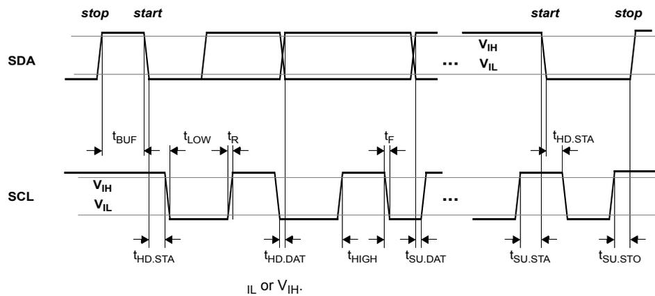
All timings are measured from either V<sub>IL</sub> or V<sub>IH</sub>.
