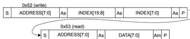
At the end of each byte, in both read and write message sequences, an acknowledge is issued by the receiving device (that is, the VL53L4CD for a write, and the host for a read).
