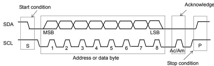
Information is packed in 8-bit packets (bytes) and is always followed by an acknowledge bit, Ac for VL53L4CD acknowledge and Am for master acknowledge (host bus master). The internal data is produced by sampling SDA at a rising edge of SCL. The external data must be stable during the high period of SCL. The exceptions to this are start (S) or stop (P) conditions when SDA falls or rises respectively, while SCL is high.
