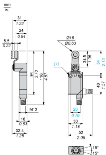
(1) 2 fixing holes Ø 4.2 mm, counterbored Ø 8 mm by 4 mm deep.
