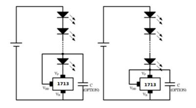
Low dropout application  $V_{PN\_Min} = 0.3V(20mA)$
