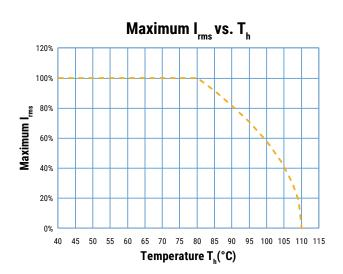
T<sub>h</sub> is the maximum ambient temperature surrounding the capacitor or hottest contact point (e.g. tracks), whichever is higher, in the worst operation conditions in °C.
