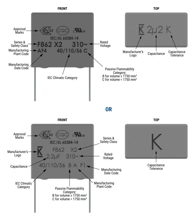
Slight change in the layout can be possible but this does not affect the content of the information of the current marking. This change will be achieved without impact to product form, fit or function, as the products are equivalent with respect to physical, mechanical, quality and reliability characteristics.
