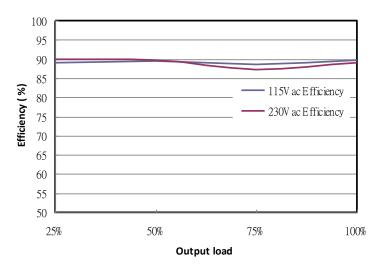
Fig. 1 Efficiency versus output load
