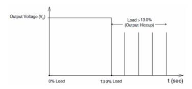
Additionally, if the lo is <130% but >110% for a prolong period of time (depending on the load), the Over Temperature Protection (OTP) will be activated due to high temperature on critical components. The power supply will then go into hiccup mode until the fault is removed; and, the input voltage is removed, then reapplied.
