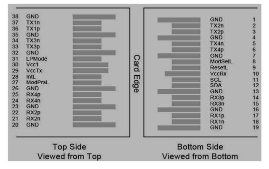
Figure 2: MSA compliant Connector
