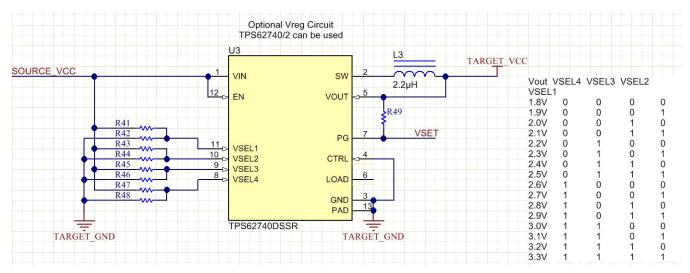
Figure 4. TPS62740 Schematic
