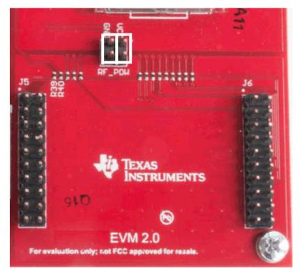
Figure 11. BoosterPack Plug-in Module Headers
