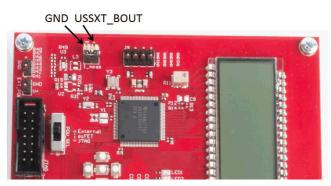
Figure 10. USSXT\_BOUT Header
