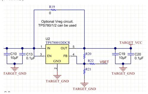
Figure 6. TPS78001 Schematic
